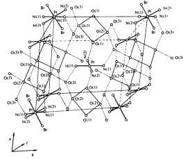
Fig. 3. Unit cell of the title compound. All the C atoms (of the diamine ligand and of the squaric acid) and some Br atoms are omitted for clarity. The hydrogen-bond network between O(3)-N(1), O(3)-O(2) and O(1)-N(2) is indicated by broken lines.
